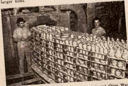
Harrop Circular Tunnel Kilo, Technical Porcelain and China Ware Corp., El Cerrito, Calif., vitreous china ware.
